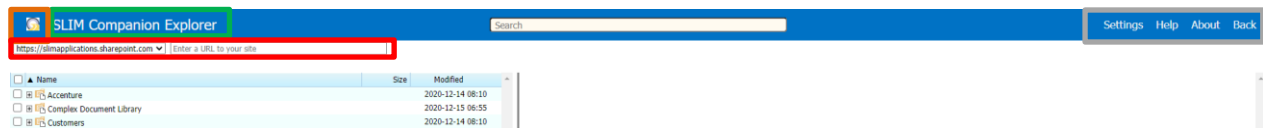
Figure 16. SLIM Companion Explorer header with the HEADERTITLE (marked in green), the HEADERLOGO (marked in amber), the HEADERMENU (marked in grey) and the HEADERSITES (marked in red).
